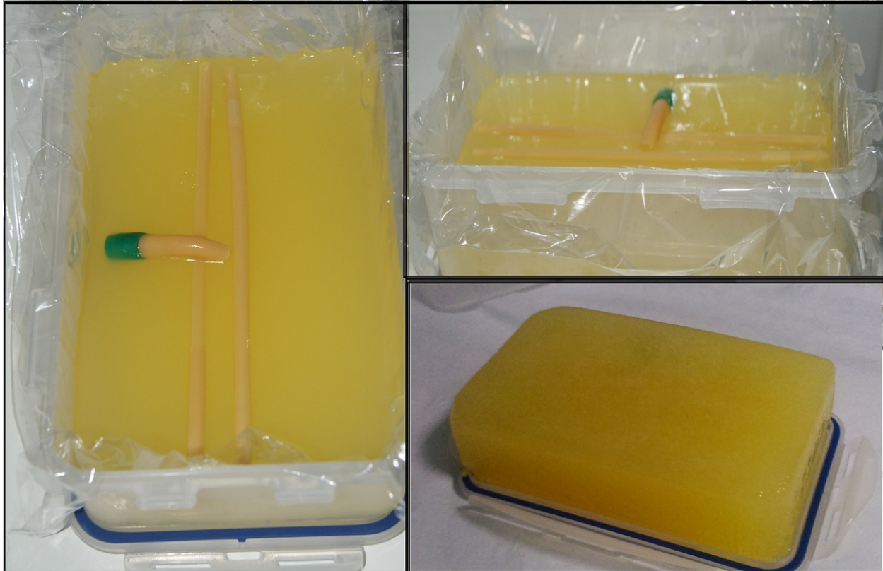
Fig. 1: Left and top right: First layer of agar-gelatin was poured in a PVC container, targets were placed on top of first layer (cling wrap was used to further removal of the phantom) Bottom right: Final product with second layer
